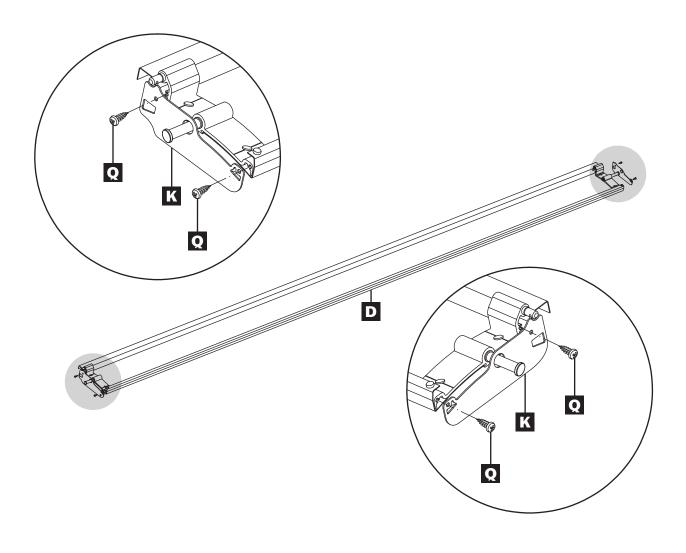
**STEP 11**Add the first louvre. Once the end baffles are connected add the remaining louvres.
