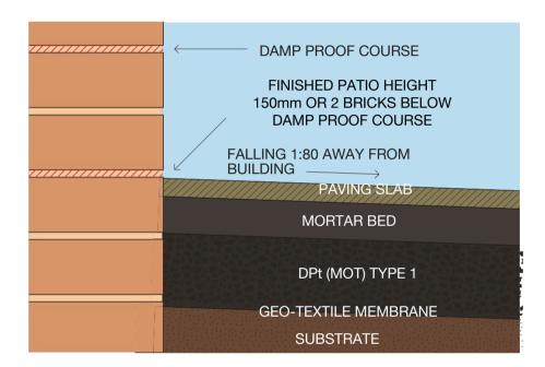
Prior to paving, drainage should always be considered. Wherever possible, drain away from the house and ensure that the finished height of the paving is 150mm or two courses below the damp proof course, unless appropriate allowances are made. Paving should be laid with a fall of 1:80. The fall needs to be applied to the excavation and the sub-base to ensure that all layers in the construction are equal.
