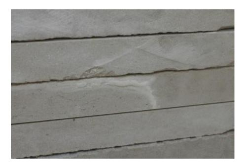
Natural stone can contain small chips which is an unavoidable part of the production process and whilst as much care as possible is taken with handling, packaging and quality control some slabs will still contain small chips. Most chips will be virtually undetectable once the stone is installed pointed and will not detract from the appearance of the finished project. Check all stone for any cracks or damage prior to installation
