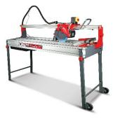
tend to be recommended for very large projects with lots of intricate cuts. The cut faster easier and with great precision. Very straight forward to use, usually they will have a Water Tray under the bed with pump feeding water directly onto the blade. As for the cutting method these would usually have either a blade capable of moving down the rail or the bed itself will slide. Some of these even come with laser levels and a perfectly straight cut.
