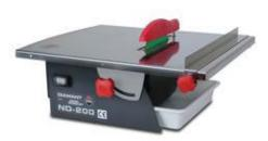
cutter and are often used when a great deal of cutting is required. These are also a more popular choice when it comes to cutting porcelain. As you can see from the image the construction is straight forward with a tray at the bottom for water. The rotating blade cuts tiles using friction whilst being water cooled.
