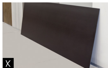
✗ Do not rest the ceramic slab on any surface without protectors.
